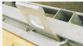
Unique cargo securement anchor point (cargo hand style) Galvanized side rails
